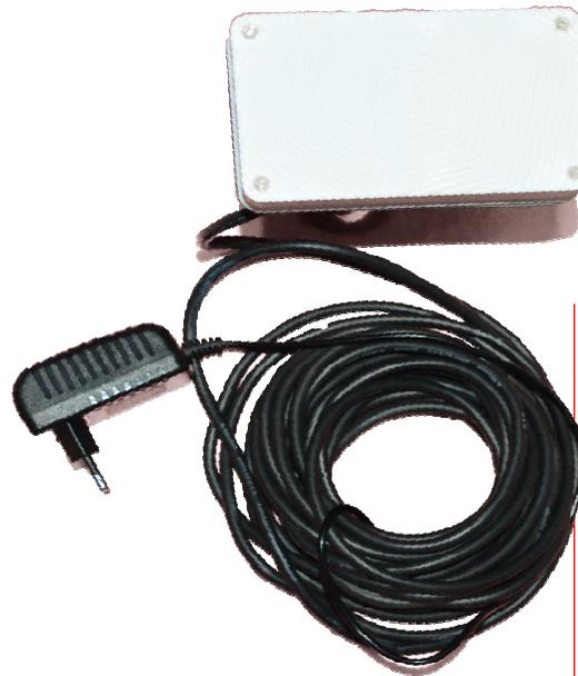
The MAM can be line-powered, or in the absence or interruption of external power. The MAM Monitor utilizes motion sensors, comparative GPS positions and custom configured sensors to gather and transmit asset status information. Each device is configured to track its asset's specific needs and provide intermediate and emergency alerts by email or text.
